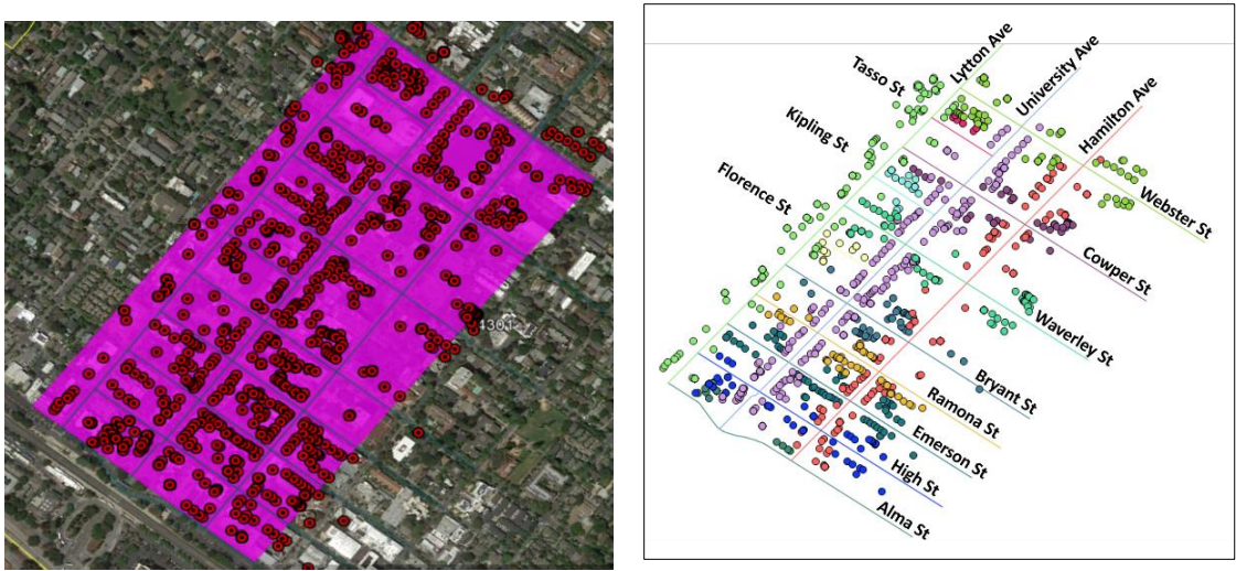
Figure 4: Downtown Palo Alto addresses in city's GIS database plotted in Google Earth and QGIS
